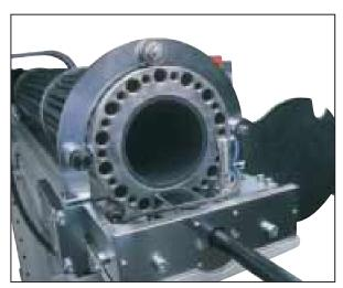
With the "Combo Barrel" you'll get superior performance that covers the total range from .039" to .500" (or .039" to .393" depending on the machine). Its reserve of 14 bars allows hours of uninterrupted, high-performance operation.
