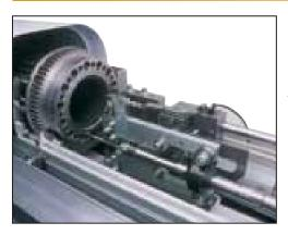
Double check remnant detection device speeds up bar end retraction for continuous production on all bar sizes.
